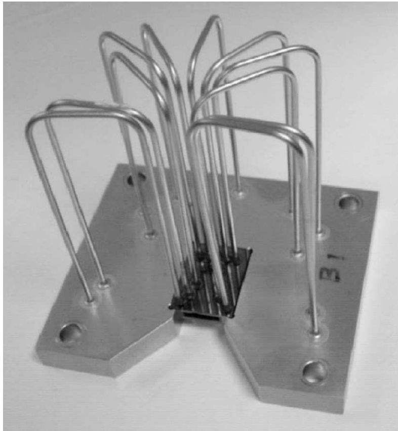
Fig. 3. Packaged microrocket die showing the 11 U-shaped stainless steel tubes that connect the silicon chip to the manifold.
