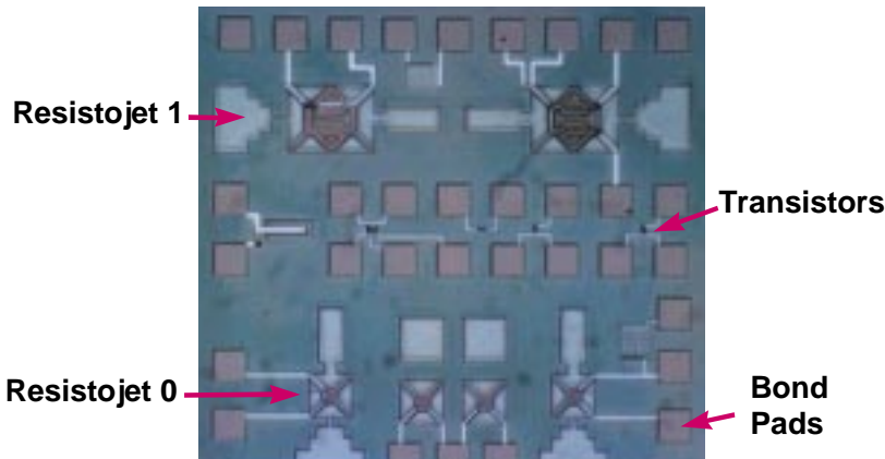
Figure 11. Photograph of an unetched silicon die with resistojet and electronic structures as received from MOSIS. (Aerospace Corp. photo)
